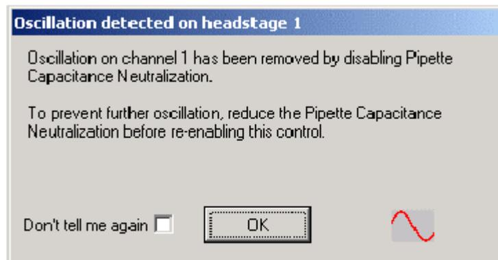
Figure 13. Oscillation detected message for I-Clamp mode.
